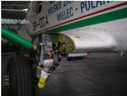
Figure 2. Adaptive Landing Gear during tests in PZL Mielec (Polish Aviation Factory) within the ADLAND project [4].
